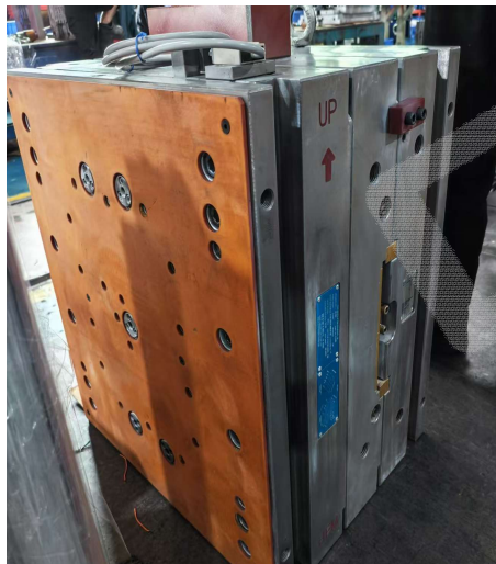
Install Nameplate and Junction Box
